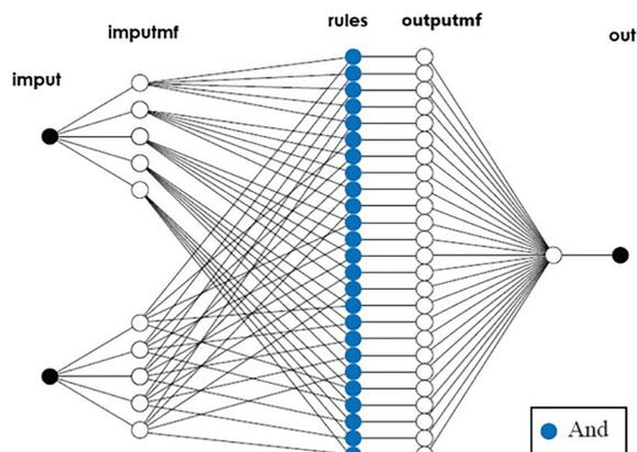
**Figure 1.** ANFIS architecture with two entry parameters and four pertinence functions.
