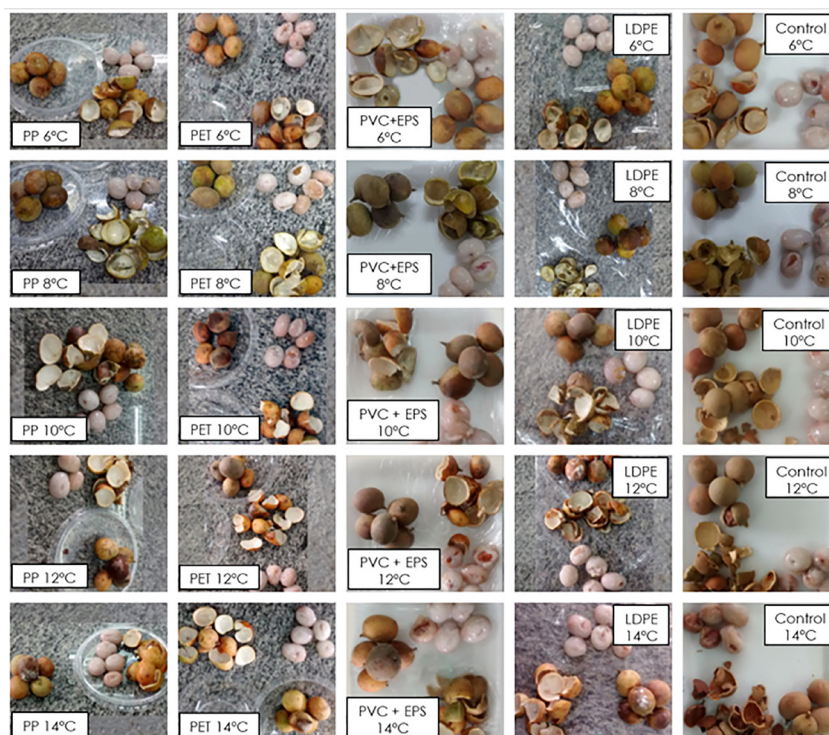
Figure 2. Aspect of pitombas packed in polypropylene (PP), polyethylene terephthalate (PET), polyvinyl chloride (PVC) + expanded polystyrene (EPS), low-density polyethylene (LDPE), and no packaging (Control) at temperatures of 6 (16 days), 8 (15 days), 10 (13 days), 12 (13 days), and 14 °C (13 days).
