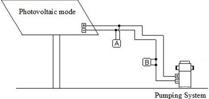
Figure 3. Layout of the system current and voltage collection system, (A) Multimeter connected in parallel for voltage measurement, (B) Multimeter connected in series for current measurement.
