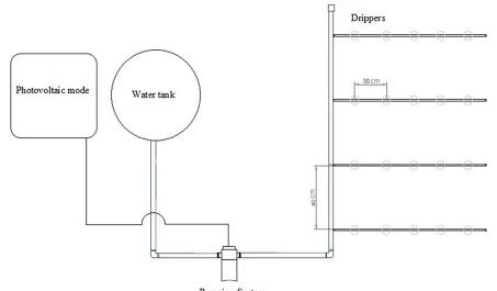
Pumping System Figure 1. Layout of the drip irrigation system with photovoltaic energy
