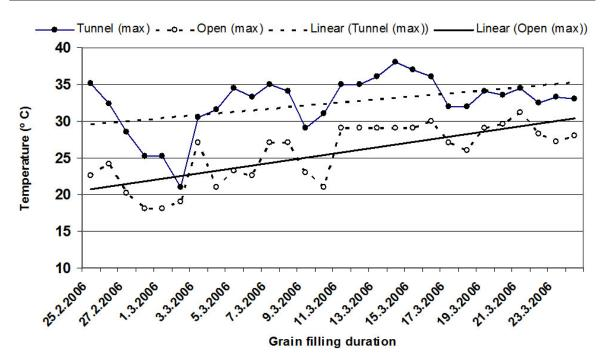
Figure 1. Difference of temperature inside the plastic tunnel and outside the tunnel during anthesis and grain filling stage.
